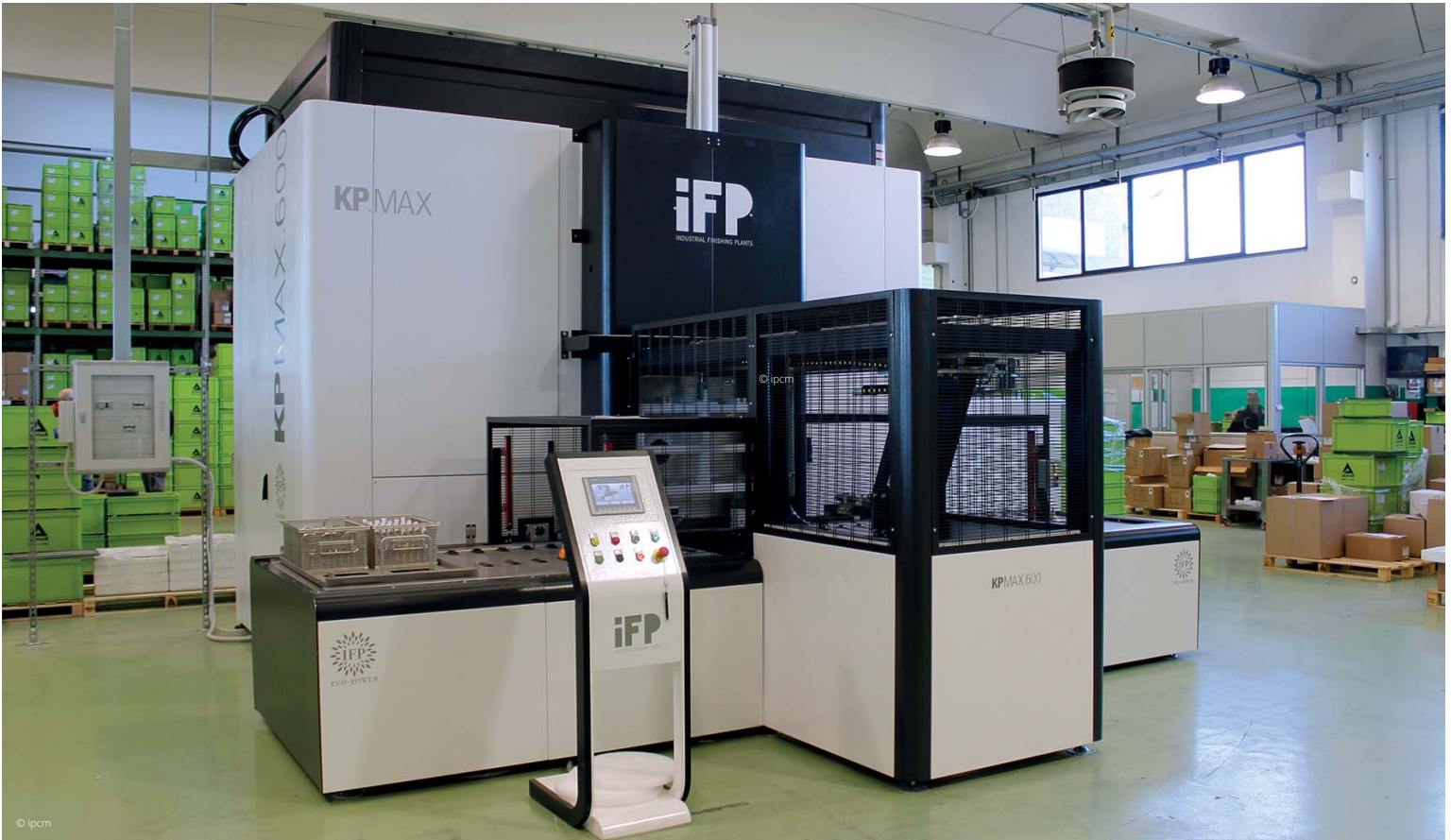
The IFP Europe KP MAX 600 cleaning plant.
