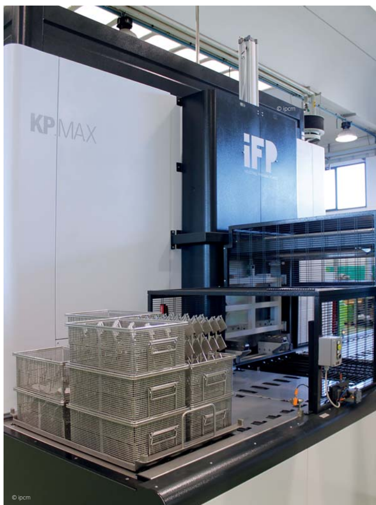
The frame on the conveyor belt can contain a maximum of 4 baskets horizontally by 3 vertically.
