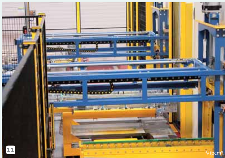
11 Both washing machines are fitted with an arm that pushes the baskets inside the washing chambers.
