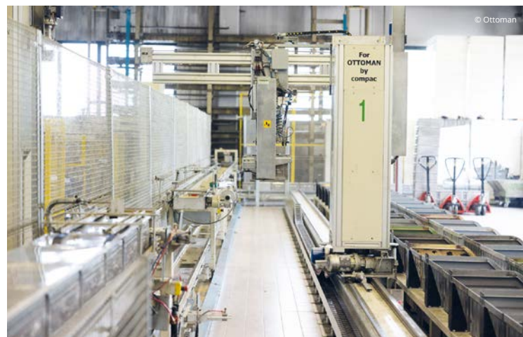
The company has equipped its entire factory with a fully automatic basket handling system.
