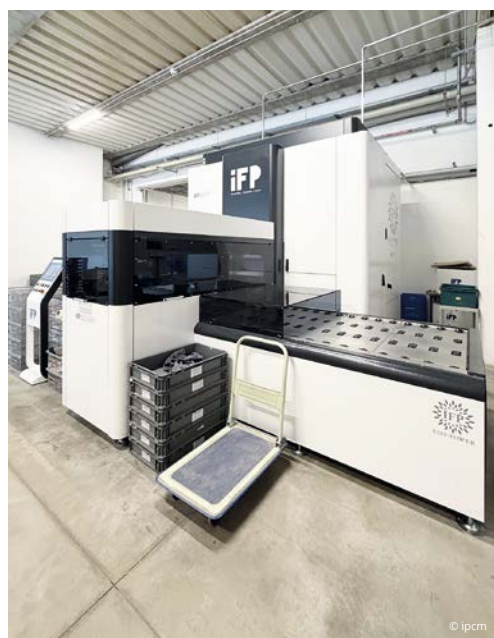
From left to right: Outside the liquid coating booth; The KP.150 Easy cleaning plant installed by IFP Europe for cleaning brass parts prior to polishing; The IFP Europe cleaning plants’ management system has been developed in line with Industry 4.0 parameters.
