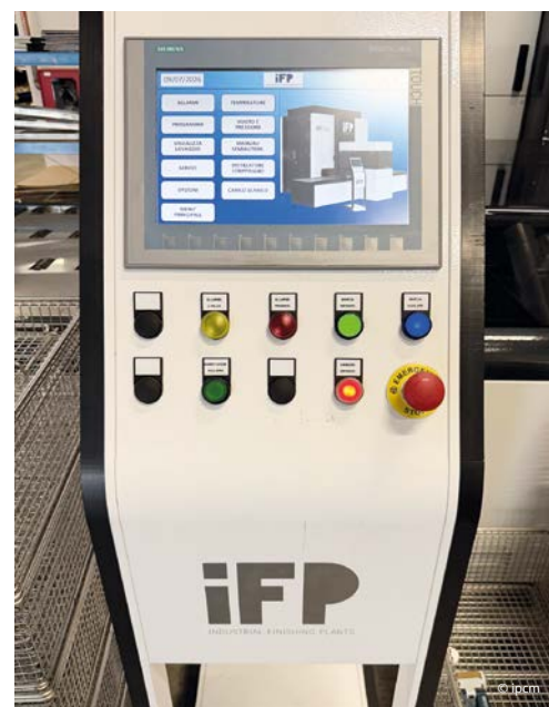
From left to right: Outside the liquid coating booth; The KP.150 Easy cleaning plant installed by IFP Europe for cleaning brass parts prior to polishing; The IFP Europe cleaning plants’ management system has been developed in line with Industry 4.0 parameters.
