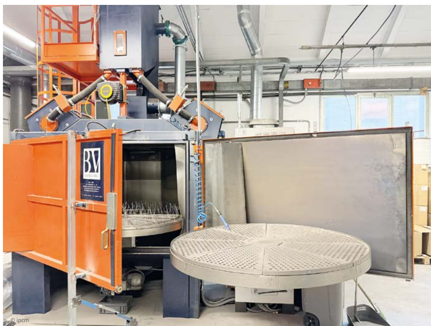
The galvanic treatment department and the shot blasting machine, where parts undergo mechanical pre-treatment before coating.
