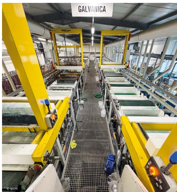
The galvanic treatment department and the shot blasting machine, where parts undergo mechanical pre-treatment before coating.
